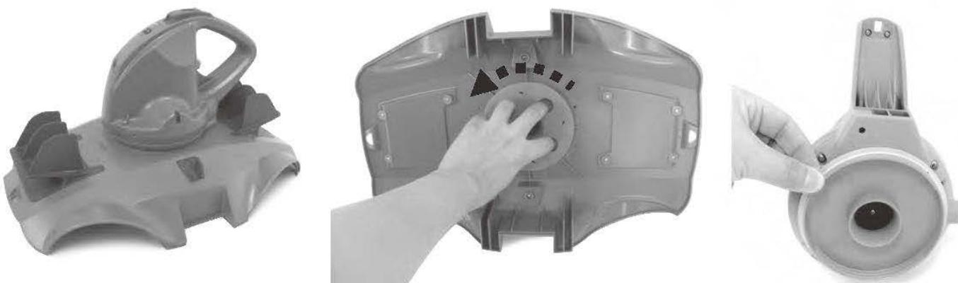
2. Use the screwdriver to unscrew the 4 screws located on the bottom of the head to release the bottom plate at first. Use the screwdriver to unscrew all the screws on the base as shown. Remove the impeller and then pry up the base and remove it to expose head inside.
